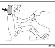
Head restraints are designed to help reduce the risk of neck injuries in case of an accident. Adjust the head restraint to the position which places the center of the head restraint closest to the top of your ears. If this is not possible for very tall passengers, adjust the head restraint as high as possible.
